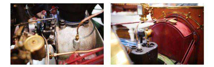
The single cylinder engine with water cooling had a displacement of 1020cc and a capacity of 10hp.
